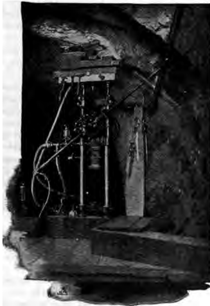
Fig 66. Sullivan Diamond Drill Drilling an Upper Hole.
